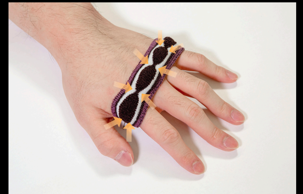
Kim et al. KnitDermis: Fabricating Tactile On-Body Interfaces Through Machine Knitting. DIS 2021
